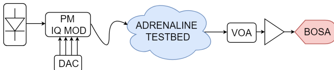
Fig. 6. Schematic diagram of the experimental setup for the high-resolution optical spectra acquisition. PM-IQ-MOD: polarization multiplexed-IQ-modulator, DAC: digital-to-analog converter, VOA: variable optical attenuator, BOSA: Brillouin optical spectrum analyser.
